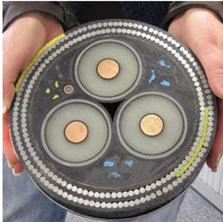
Cross section of a 132 kV cable
